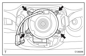
(b) Disengage the 4 screws and remove the spiral cable.
